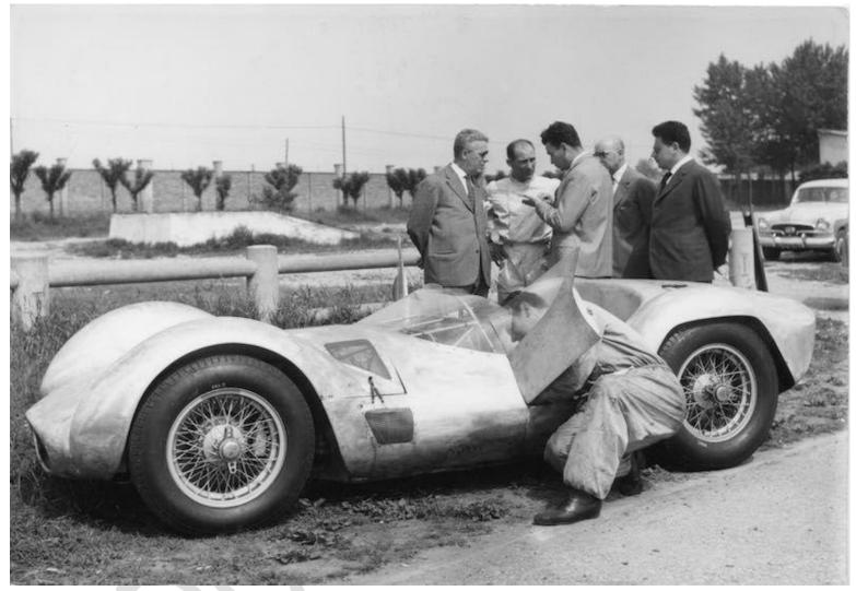
And a most inspired gamble it was: take a chassis of intricate, thin-gauge tubing that truly resembled a birdcage; mate an upswept duck-butt tail to front clamshell fenders; fire the whole shooting match with a zooty four-cylinder Maserati that sounds just a Meyer-Drake Offenhauser, but minus all that high-revving Ferrari rigmarole of a Ferrari – this was Maserati's great invention, the Birdcage.
